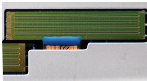
Figure 8. Detail of an HP Thermal Inkjet die
